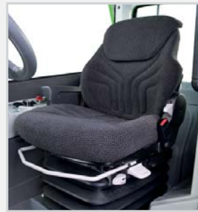
Pneumatic seat for improved comfort.
