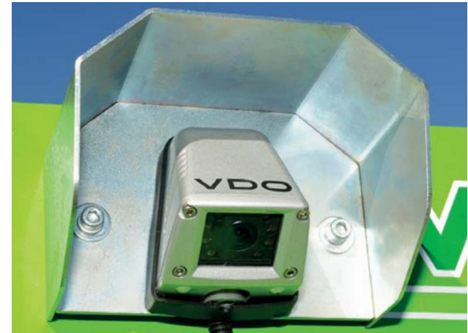
Rear exterior camera (optional) let you see behind the telehandler, and it is automatically activated with the reverse gear to be shown on CDC Display
