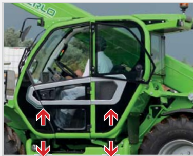
CS hydropneumatic suspended cab which can be activated by the operator. The only one of its kind on the market.
