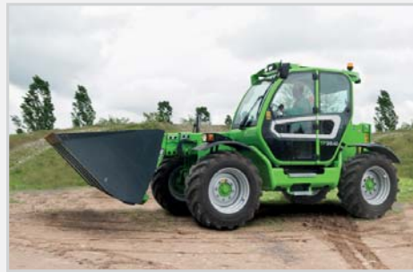
BSS hydropneumatic suspension of the boom (optional), which can be activated by the operator, automatically deactivates under 3 km/h to ensure maximum precision in the positioning of the loads.
